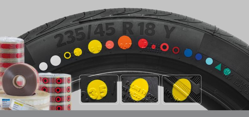
tire\_dots are heat activated transfer labels for marking of vulcanized rubber tire sidewalls. They identify various tire parameters including 1st harmonic, imbalance, conicity or may be used to support internal sorting processes. Like a skin, the elastic tire\_dots adopt the surface contour of a vast majority of challenging sidewall structures.
